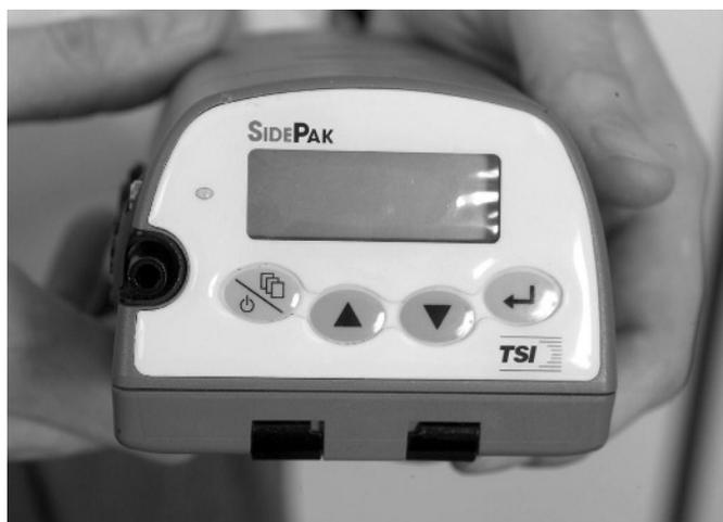
**Figure 1** The TSI SidePak AM510 Personal Aerosol Monitor.
