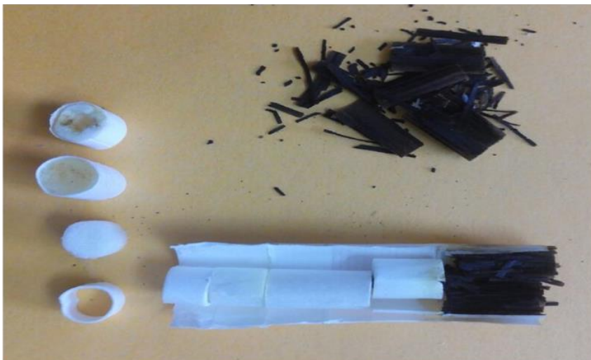
Fig. 11 Changes in the structure of the component sticks after the smoking session under the influence of temperature of the heater
